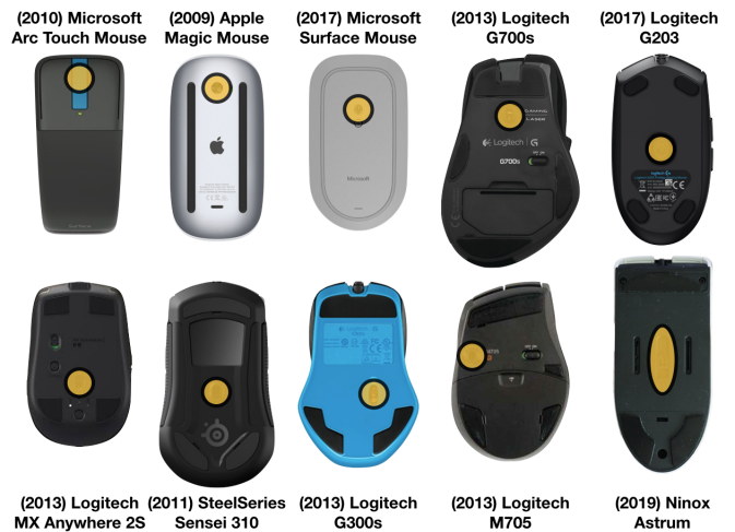
Figure 2. Commercial mice (shown to scale) exhibit a wide distribution of displacement sensor designs. Note that Ninox Astrum is equipped with a slider for a variable sensor position.
